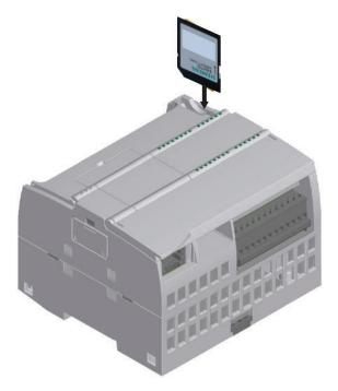
To insert a memory card, open the top CPU door and insert the memory card in the slot. A push-push type connector allows for easy insertion and removal. The memory card is keyed for proper installation.
